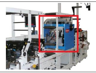
Off-line units (page 12 to 13), standalone units for the production of selfadhesive rolls to feed existing presses;
